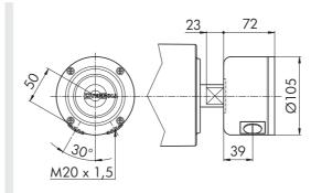
Fig.: DM 0113, terminal box, technopolymer
