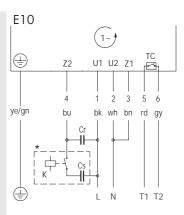
Fig.: 1-phase, 7-core cable
