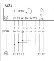
Fig.: 3-phase, 7+2 core cable, winding for 2 voltages, delta connection
