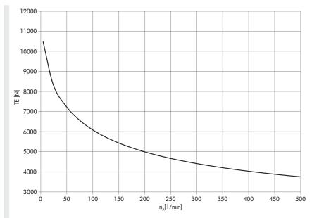
Note: The correct value for the maximum permissible belt tension is determined from the speed of the drum motor. When selecting the motor, also check whether the maximum permissible TE value fits the desired drum width (FW).
