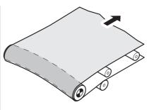
Fig.: Damaged drum motor due to over-tensioning
