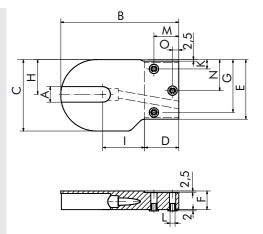
Fig.: Right bracket (A) aluminum or VA with cable connection slot Fig.: Right bracket (A) PE for drum motor with cable connection slot
