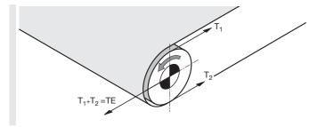
The required belt tension T1 (top side) and T2 (bottom side) can be calculated in accordance with DIN 22101 or the CEMA standard. Based on the information from the belt manufacturer, the actual belt tension can be roughly determined by a measurement of the belt elongation during tensioning.
