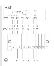
Fig.: 3-phase, winding for 2 voltages, star connection
