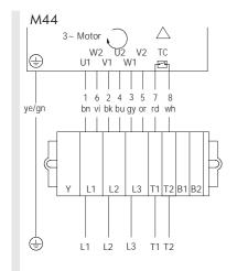
Fig.: 3-phase, winding for 2 voltages, delta connection
