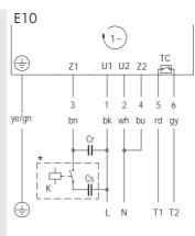
Fig.: 1-phase, 7-core cable
