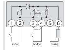
Fig.: Half-wave rectifier
