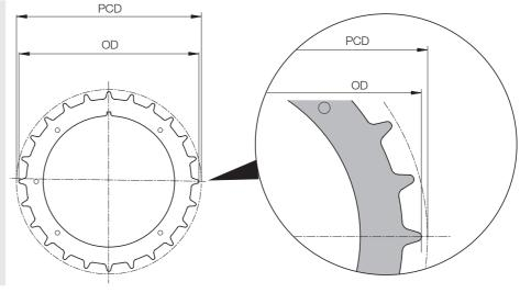
OD = Outer diameter in mm PCD = Pitch circle diameter in mm
