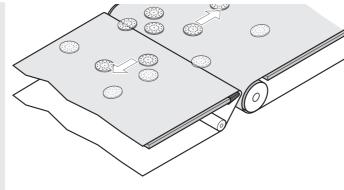
Fig.: Knife-edge conveyor
