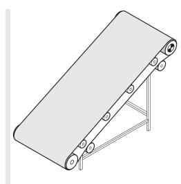
Fig.: Inclined conveyor
