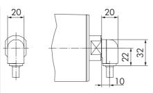
Fig.: Elbow connector, Technopolymer
