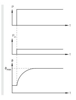
The majority of Interroll Drum Motor windings with an efficiency of over 50 % are suitable for operating mode \$1 and continuous running duty. Please refer to the electrical data tables for standard motors and motors for applications with positive drive belts or no belts. The value is listed with the symbol n for efficiency.
