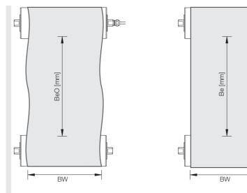
Fig.: Measuring the belt elongation
