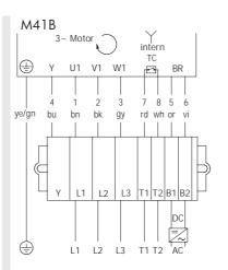
Fig.: With brake, 3-phase, winding for 1 voltage, star connection
