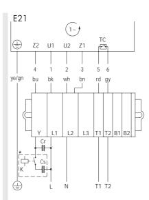
Fig.: 1-phase, 7-core cable
