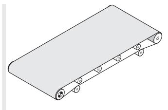
Fig.: Roller bed conveyor
