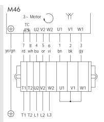
Fig.: 3-phase, 7+2 core cable, 2 speeds, double-star connection
