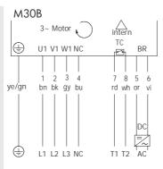
Fig.: With brake, 3-phase, 7+2 core cable, winding for 1 voltage, delta connection
