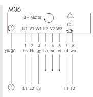
Fig.: 3-phase, 7+2 core cable, 2 speeds, delta connection
