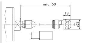
Fig.: Mounting dimensions with a mounting tool
