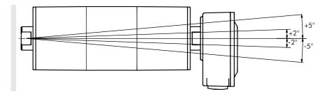
All drum motors must be mounted within  $\pm 5^{\circ}$  of the horizontal.
