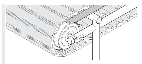
Fig.: Open conveyor design for hygienic cleaning
