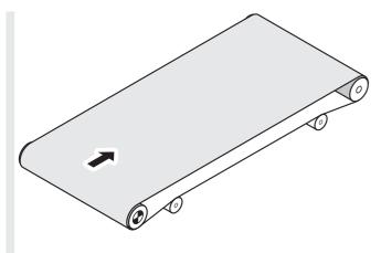
Fig.: Short friction drive belt conveyor with tail drive
