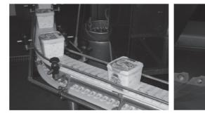
Modular plastic belts, solid homogeneous belts, steel mesh or wire belts are positively driven, i.e., with no belt tension. Since the belt has hardly any direct contact with the drum shell, the heat dissipation is less effective in these applications. For this reason, the drum motor should be used with a frequency inverter that is optimized for this application.
