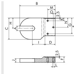
Fig.: Right bracket (A) aluminum or VA
