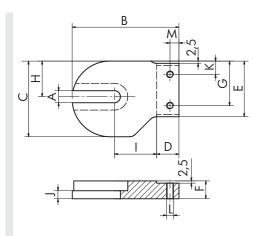
Fig.: Right bracket (A) aluminum or VA
