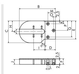
Fig.: Right bracket (C) aluminum or PE
