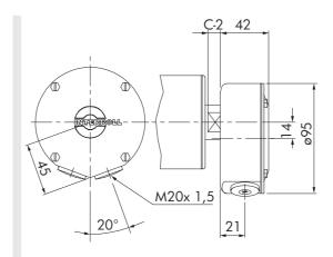
Fig.: Terminal box, stainless steel
