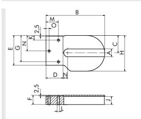
Fig.: Left bracket (B) aluminum or PE
