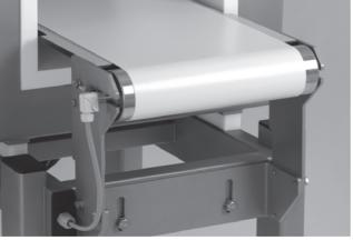
Friction drive belts are driven via the friction between drum motor and conveyor belt. The drum motor is normally crowned to prevent belt wander. The belt must be tensioned in order to transfer the torque from the drum motor. The top surface of the belt can be flat, plain or have a ribbed, grooved or diamond pattern.
