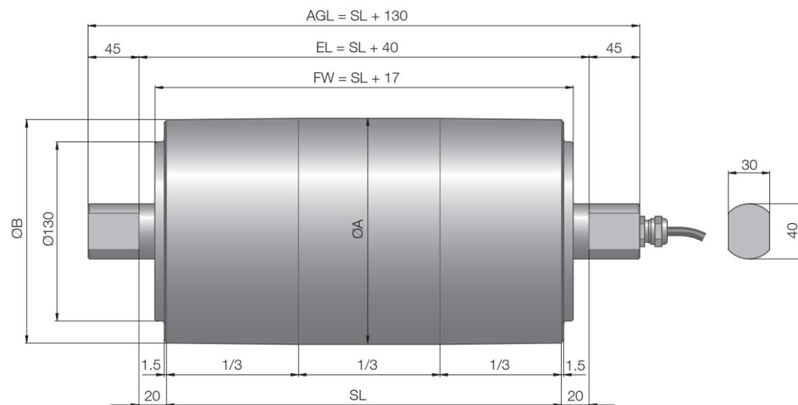
Fig.: Drum motor with straight connector
