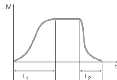
**Fig.:** Closing and opening response time
