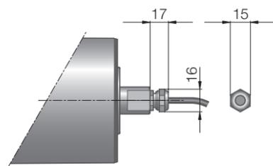
Fig.: Straight connector, brass/nickel
