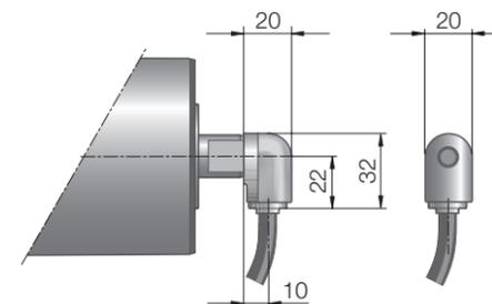
Fig.: Elbow connector, technopolymer
