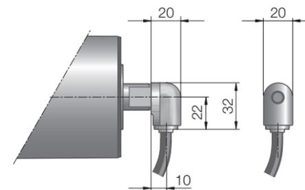
Fig.: Elbow connector, technopolymer
