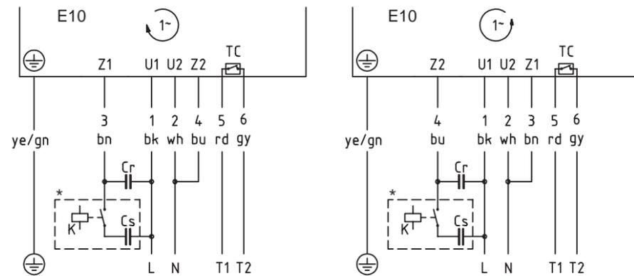
**Fig.: 1-phase operation, 7 lead cable**
