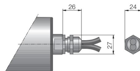
Fig.: Straight connector / Feedback device,
