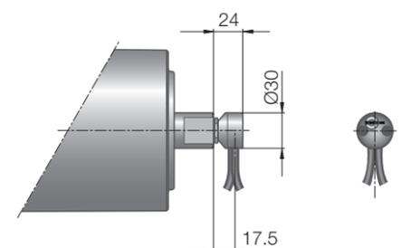
Fig.: Elbow connector / Feedback device,
