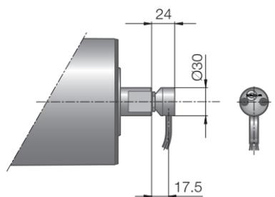
Fig.: Elbow connector, stainless steel
