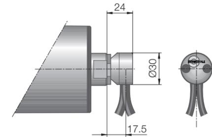
Fig.: Elbow connector / Feedback device, stainless steel
