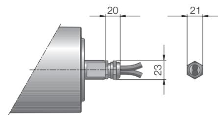
Fig.: Straight connector / Feedback device,
