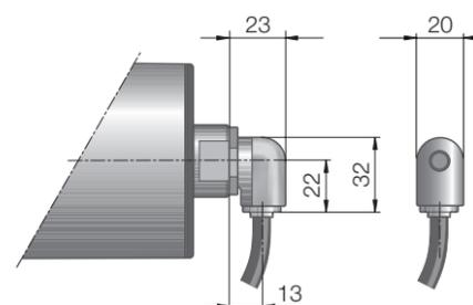
Fig.: Elbow connector, technopolymer
