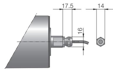
Fig.: Straight connector, stainless steel
