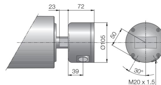
Fig.: Terminal box, technopolymer
