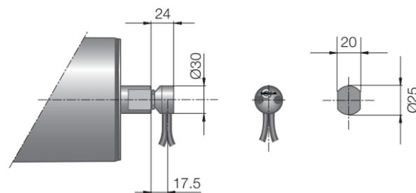
Fig.: Elbow connector / Feedback device, stainless steel
