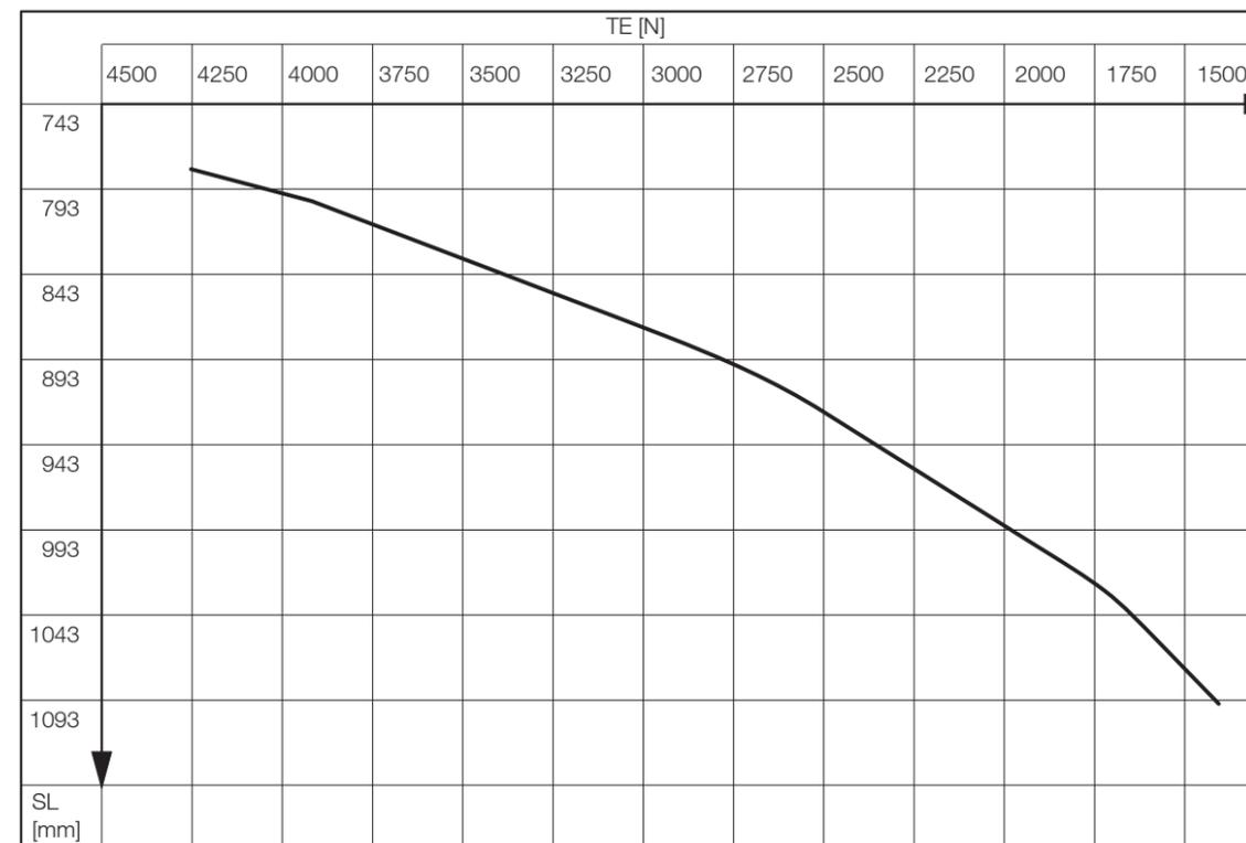
**Note:** To get the right value of the maximum allowed belt tension, first find the maximum allowed TE value for the drum motor RPM. For motors with SL > 750 mm, check if the maximum allowed TE value for the SL is lower. In this case, use the lower value as maximum allowed TE value.
