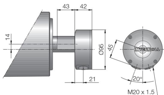
Fig.: Terminal box, stainless steel
