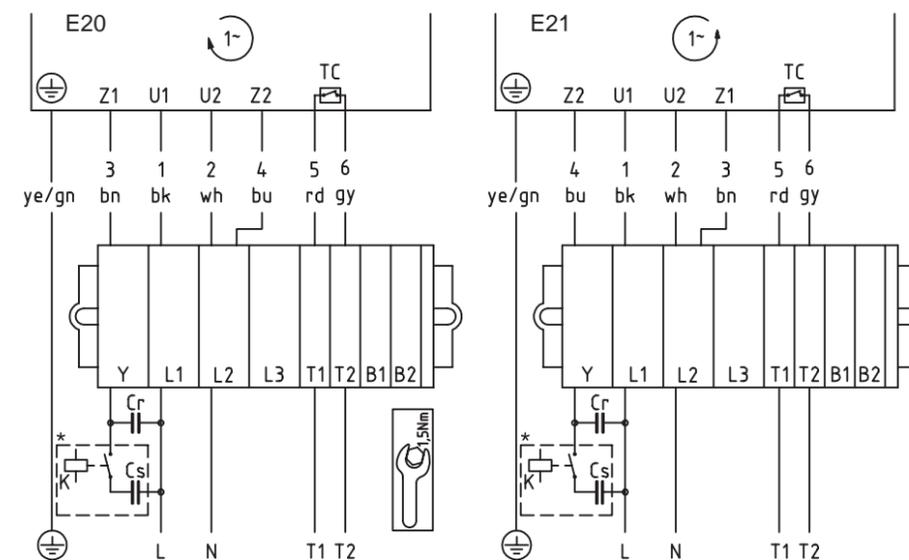
**Fig.: 1-phase operation, 7 lead cable**
