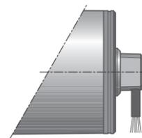
Fig.: Shaft cap with cable protection, aluminium
