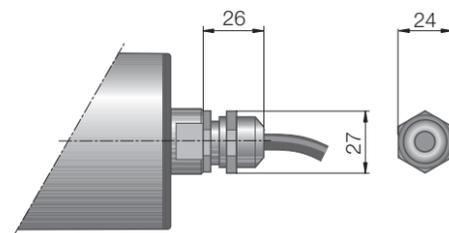
Fig.: Straight connector, brass/nickel or stainless steel
