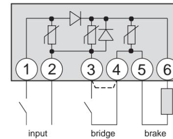
Fig.: Half-wave rectifier
